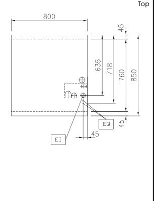
Electric Supply voltage: 400 V/3N ph/50/60 Hz Electrical power, max: 12 kW **Key Information:** 100 °C **Working Temperature MIN:** Working Temperature MAX: 450 °C External dimensions, Width: 800 mm External dimensions, Depth: 850 mm External dimensions, Height: 250 mm Net weight: 120 kg Configuration: One-Side Operated;Top Front Plates Power: 3 - 3 kW **Back Plates Power:** 3 - 3 kW Solid top usable surface 670 mm (width): Solid top usable surface
